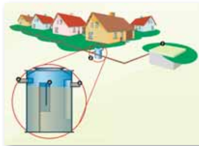
Fat separator (at the grease source)
